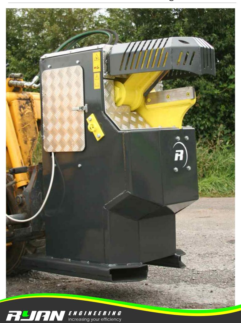
Removable Panels. These scratch resistant panels are fitted to high wear areas, increasing durability and ensuring the shears will look like new for many years.
