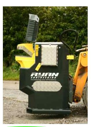
Cobra Shears are powered by hydraulic cylinder connected to various power source, such as bob cat, tractor etc.
