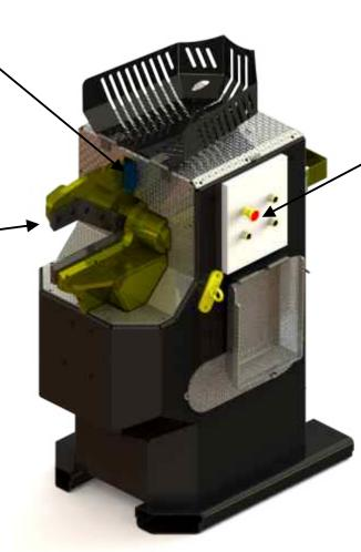
Control panel. The shears are operated from this panel. The panel also allows the operator to switch between automatic and manual jaw opening.
