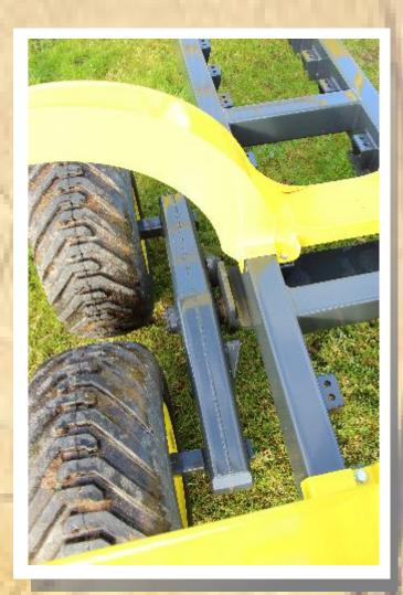
Adjustable bogie axles can be moved to optimize the turning radius specific to your load size and forest conditions.
