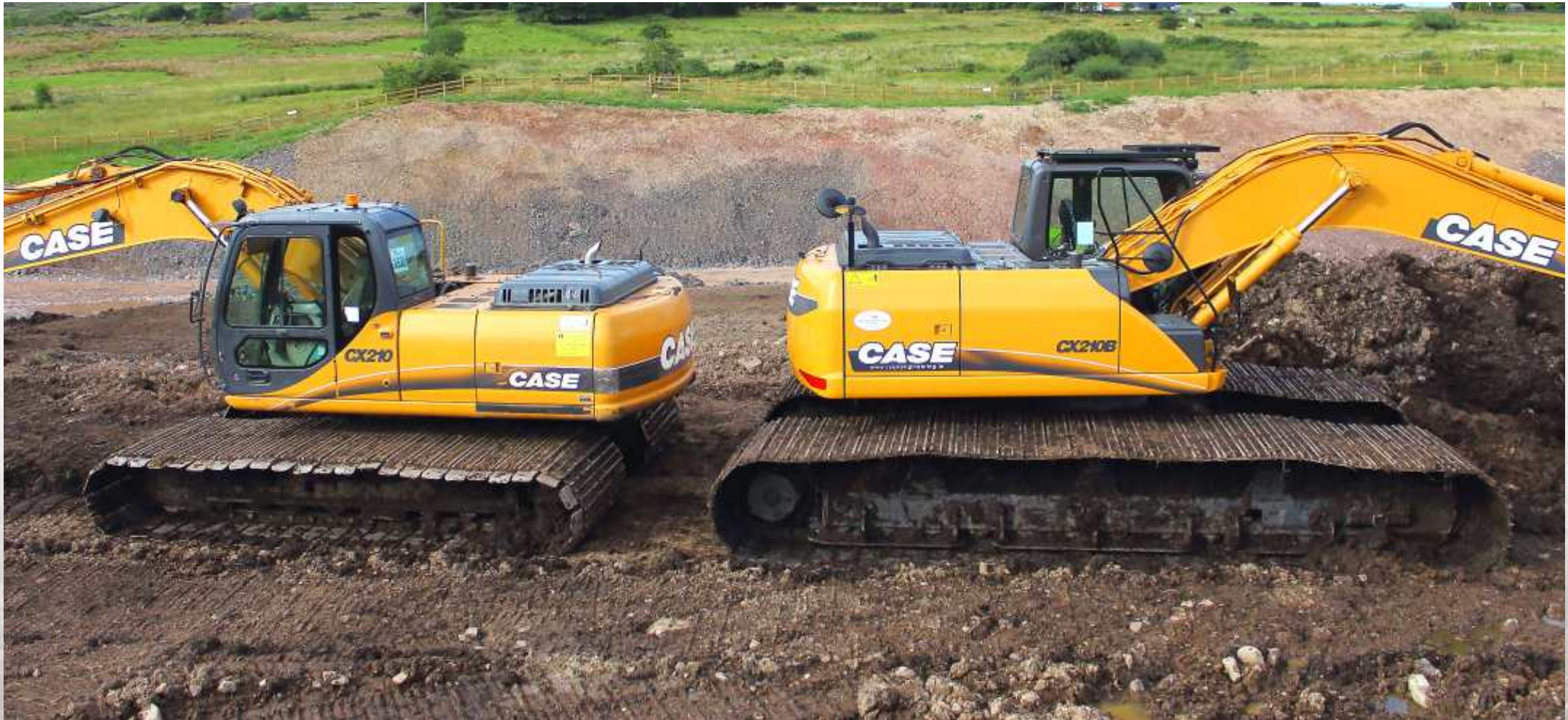
21 tonne excavator modified standard undercarriage
